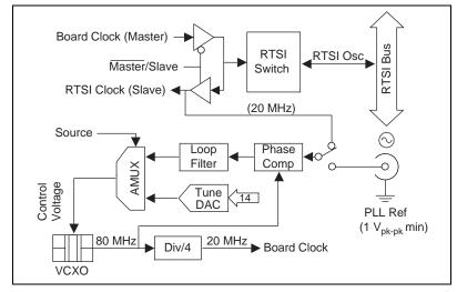
Figure 2-11. PLL Architecture for the NI 5401 for PCI
